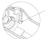
Bridge clamp strain relief can be snapped into the lower part of the housing for easier installation. For disassembly, the side lugs must be operated with a slot screwdriver
