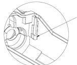
Bridge clamp strain relief can be snapped into the lower part of the housing for easier installation. For disassembly, the side lugs must
